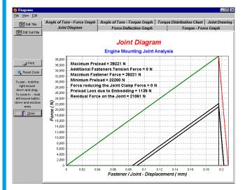
If a joint is being designed the program can estimate the size of bolt required for the application. Once the bolt size has been estimated, or details of an existing joint have been entered, detailed calculations can be performed. The calculations will determine whether or not the bolt will fail by:
