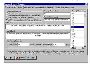
The program accesses extensive databases on thread sizes, bolt material properties, thread and head friction coefficients and torque tables. The program works in both metric and inch based units and associated thread and bolt material data.
