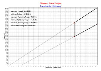
The program includes extensive databases of friction values (anticipated maximum and minimum values derived from test results). The program can use this data to establish the likely scatter in the bolt preload to allow the analysis to be completed on the basis of minimum preload values rather than the mean or maximum.
