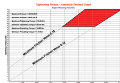
The effect of friction on bolt preload
