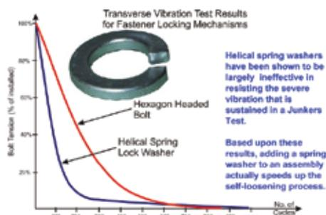
Placing a helical spring washer under the bolt head has been shown on some tests to speed up the loosening, others show that the use of such washers give a similar performance to using a bolt without any locking device. Many large OEM manufacturers are aware of these findings and no longer specify such washers in their internal standards. However, judging by the continued use of these washers, many organisations do not seem to be aware of these findings.
