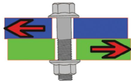
Transverse movement of a bolted joint
