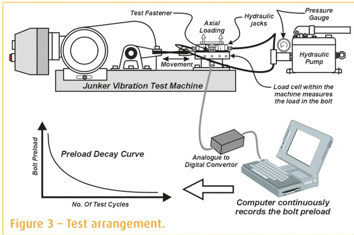
Figure 3 – Test arrangement.
