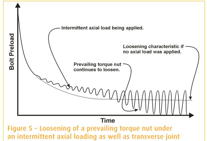
Figure 5 – Loosening of a prevailing torque nut under an intermittent axial loading as well as transverse joint
