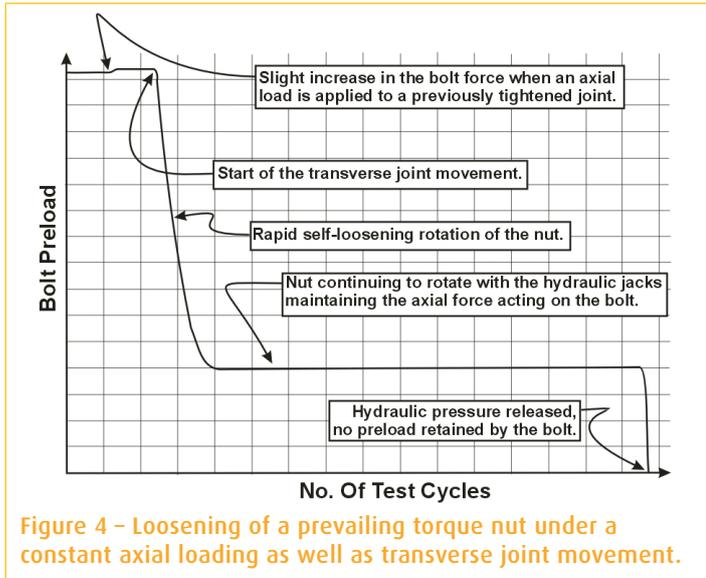
Figure 4 – Loosening of a prevailing torque nut under a constant axial loading as well as transverse joint movement.
