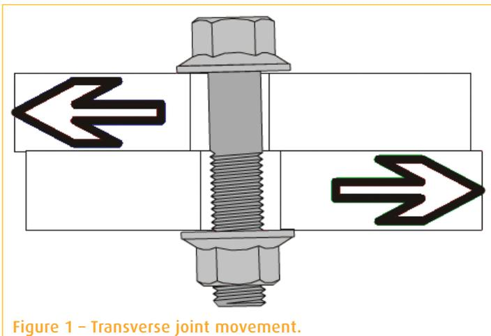
Figure 1 - Transverse joint movement.
