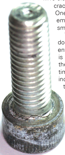
Figure 1: M10 electroplated 12.9 screw cracked under the head
